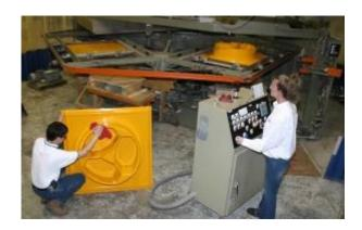
**Thermoforming:** The thermoforming process involves preheating a flat sheet of plastic, then bringing it into contact with a mold—taking on that shape. This "forming" is accomplished by vacuum, pressure and/or mechanical force.
